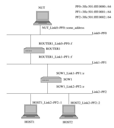
Fig. 2 Topology for End-Node: Tunnel mode with SGW
