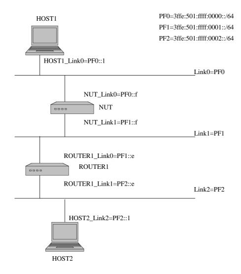
Fig. 3 Topology for SGW: Tunnel mode with End-Node
