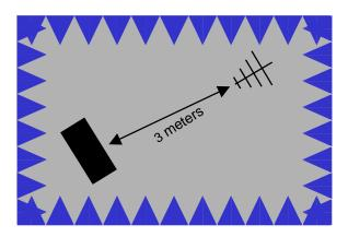
The following table shows the FCC Class B limits and CISPR-22 Class B Limits. The perenthised numbers show the same limit with the 6dB offset added to compensate for the three to ten meter difference.
